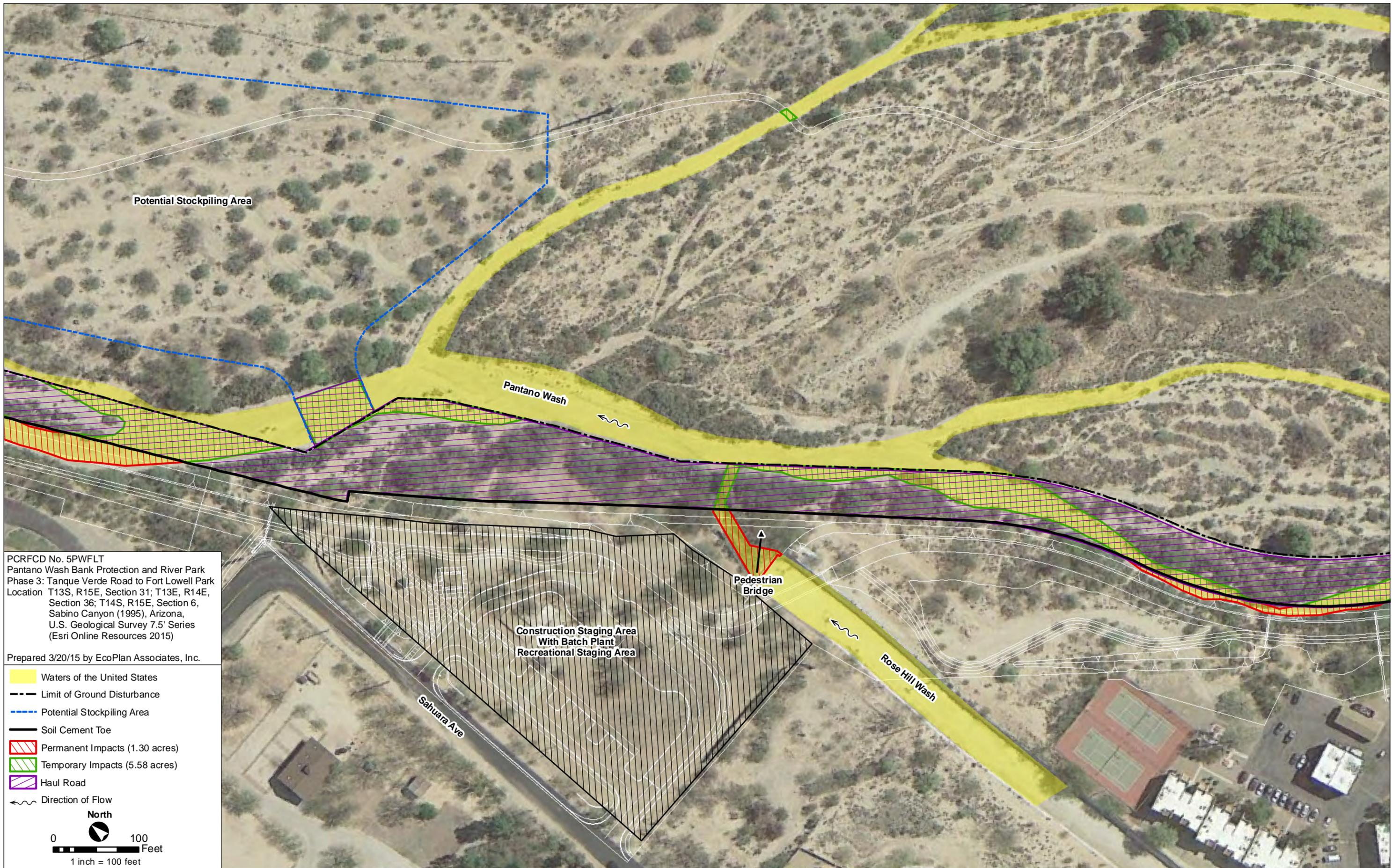
Figure 5. Permanent and temporary impacts to Waters of the United States at Pantano Wash and Rose Hill Wash, near Sahuara Avenue and the proposed recreational staging area
